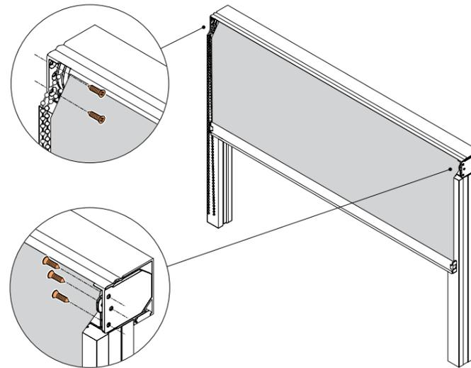
c) Lift the rail in place between screen guides.
