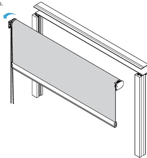
b) Fix the screen into the frame with 2 screws at ball chain mechanism and 3 screws at spring end.
