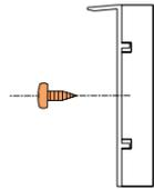
Fit screen guide timber to screen guide extrusion and fit seals. Fit the larger seal to the exterior.
