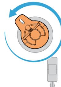
c) Push remaining length of spring into screen roll.
