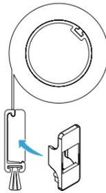
Centre extrusion with timber – approx. 30mm from either end. Screw screen cover timber to screen cover extrusion.
