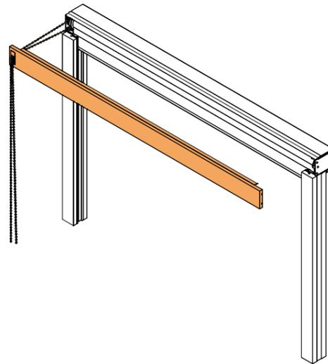
c) Operate the screen fully to ensure the ball chain joiner won't become lodged in the top guide. If it does, pull screen tube out and reposition the ball chain and the sprocket.
